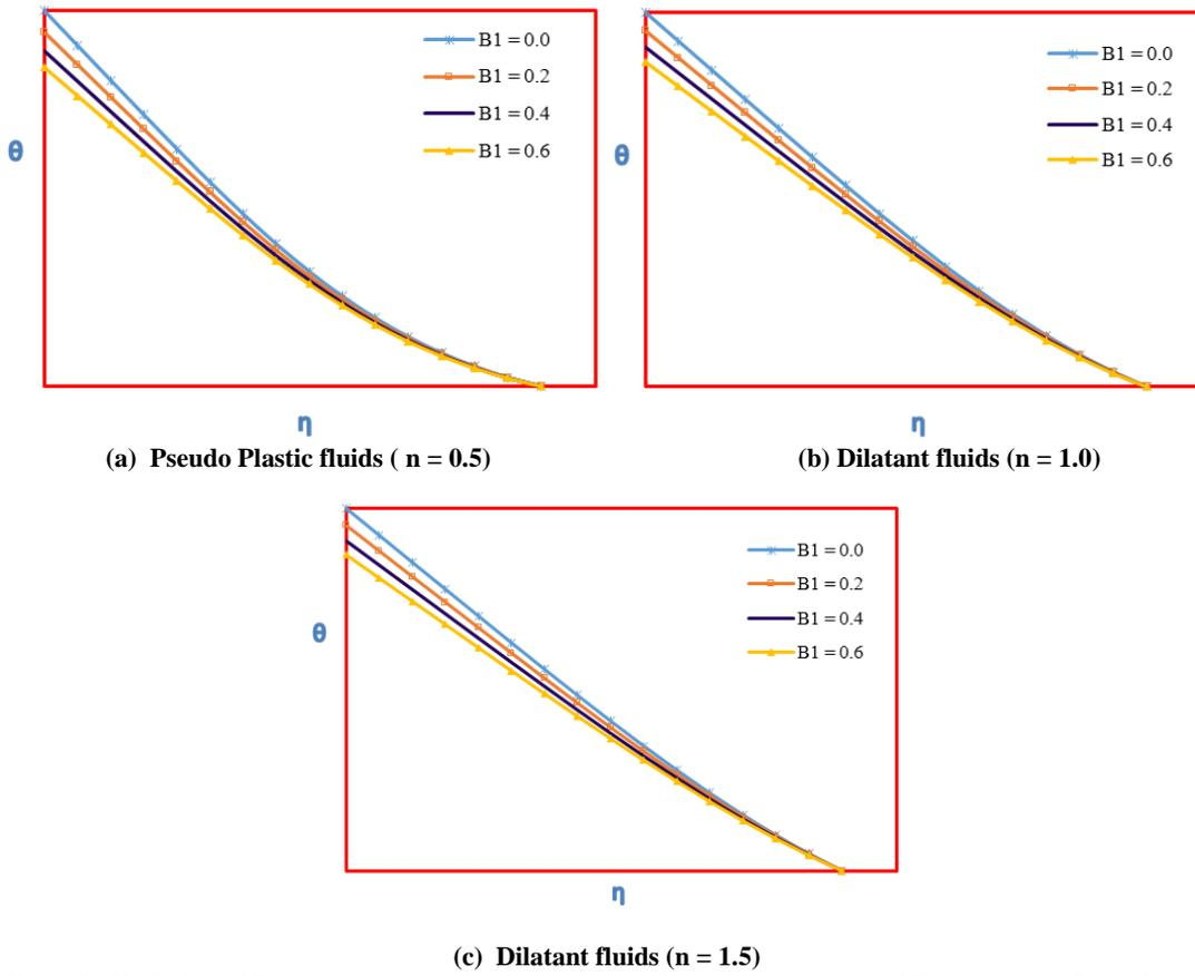
Figure 2. Variation of Temperature profiles for various values of Temperature Slip parameter  $B_1$  with  $M = 0.2$ ,  $Pr = 0.7$ ,  $Le = 1.0$ ,  $Sr = 0.04$ ,  $Du = 0.02$ ,  $A_1 = 0$ ,  $C_1 = 0$ .
