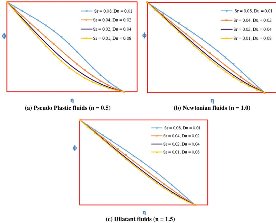
Figure 5. Variation of Concentration profiles for various values of Soret number and Dufour number with  $M = 0.2, Pr = 0.7, Le = 1.0, A_1 = 0, B_1 = 0, C_1 = 0$ .
