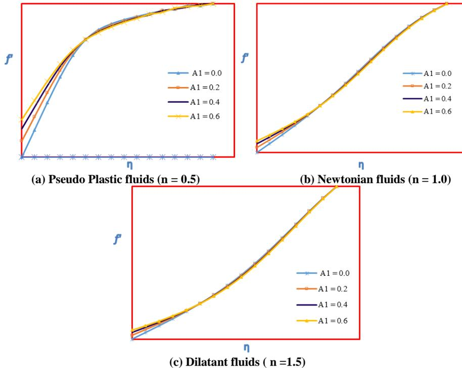
Figure 1. Variation of Velocity profiles for various values of Velocity Slip parameter  $A_1$  with  $Pr = 0.7$ ,  $Le = 1.0$ ,  $Sr = 0$ ,  $Du = 0$ ,  $M = 0$ ,  $B_1 = 0$ ,  $C_1 = 0$ .
