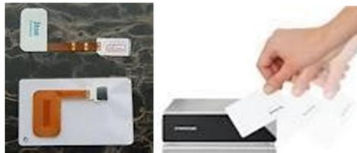
Fig.3a RFID tag Fig.3b RFID card and reader
