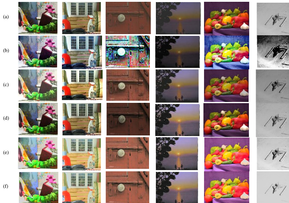
Figure 2. Restored image by different methods (a) Original Image (b) Histogram equalization method(c) Method (d) V-transform method (e) Proposed method. (f)(Proposed method with sharp filter.
